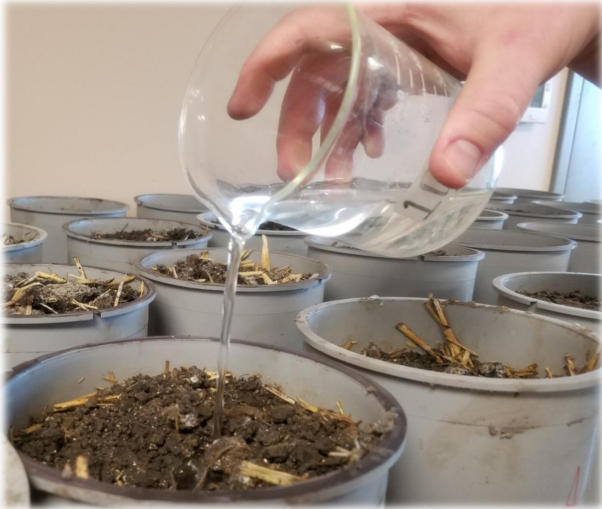
Weekly watering to simulate natural precipitation
