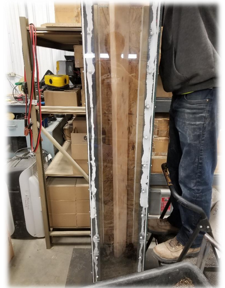
Attaching Plexiglass Front
