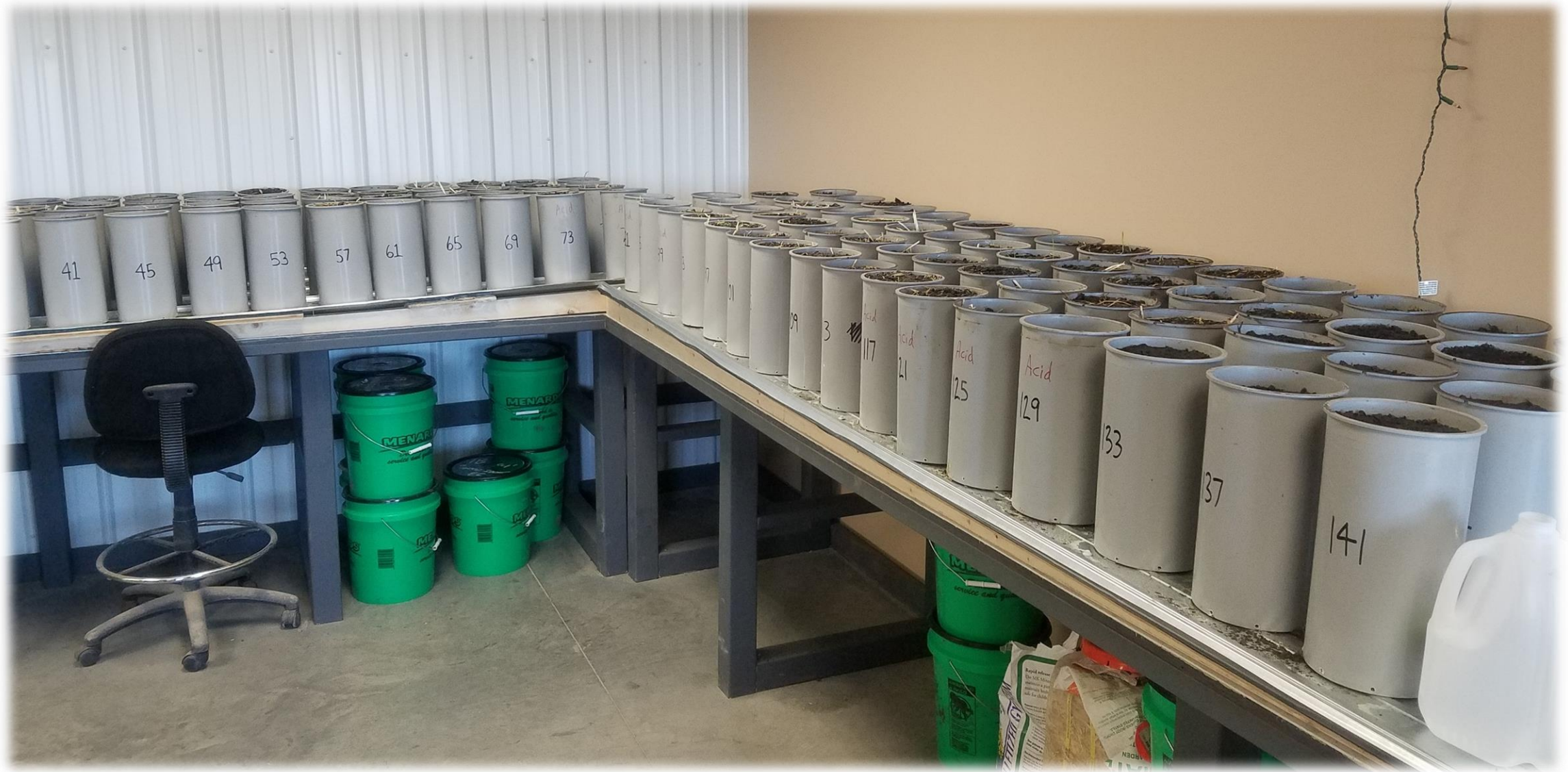
Test Cells with Drainage for Water Collection
