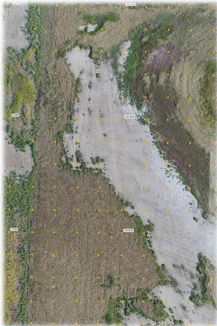
EC Test Grid (20' on Center)
