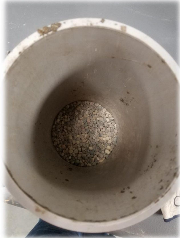
Pea Gravel as Drainage Layer
