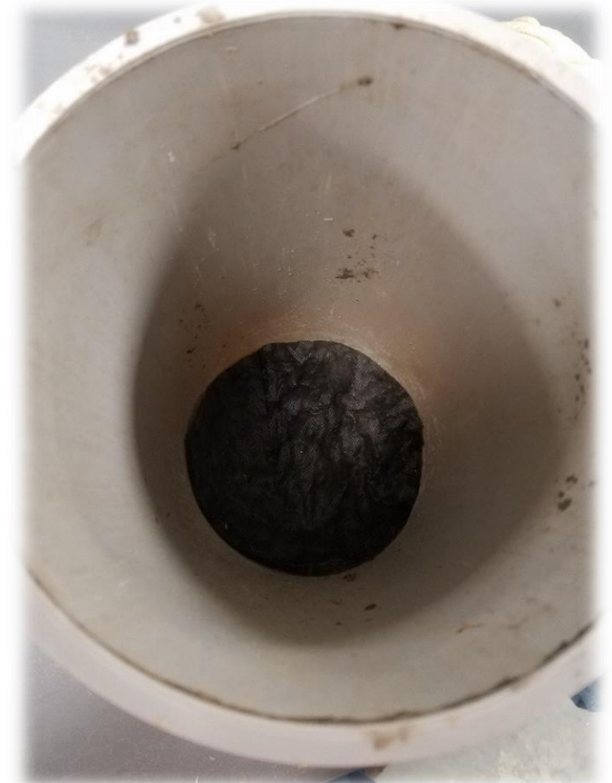
Filter Fabric Between Gravel and Amended Soil
