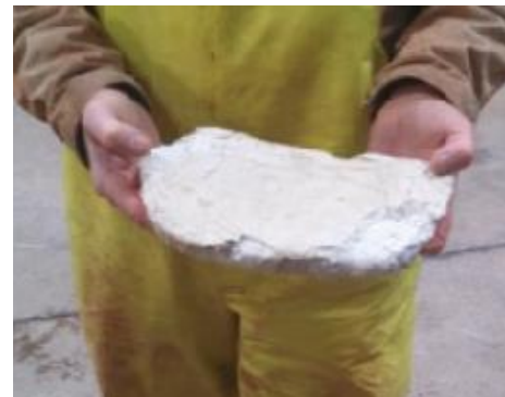
Salts Solidified and Stabilized for Disposal
