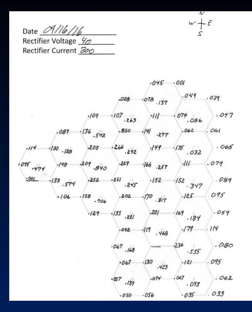
Current measurements were made at each electrode during operations help identify bad electrodes and general operating uniformity. (Readout is amps/100)
