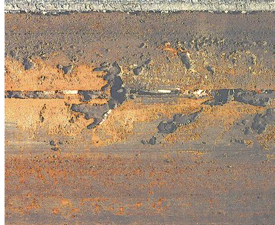
corrosion in tubing exacerbated by abrasion from wireline operators.
