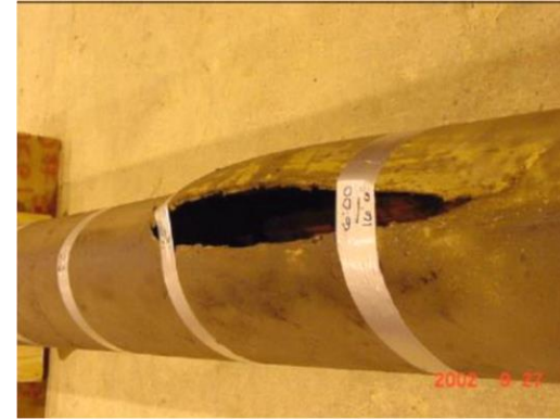
Burst – Above cement support
