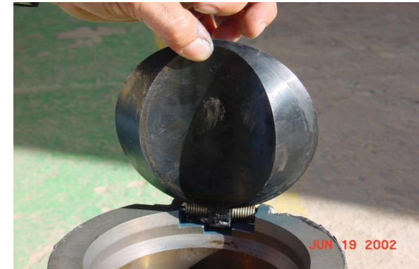
Right top: plug valve – common in surface treating “iron”
