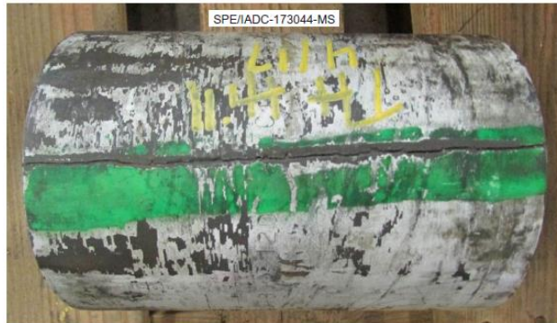
Hydrogen embrittlement – high strength P-110 Coupling
