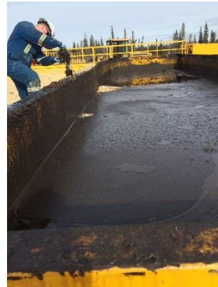
OBM & Cuttings Exit Shale Shakers
