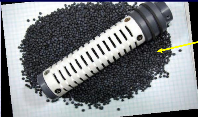
Bio-Trap® Sampler with Bio-Sep® Beads
