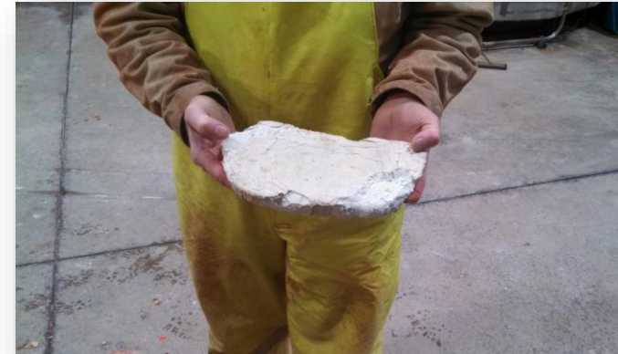
To pass TCLP, salt slurry resulting from concentrating Marcellus shale produced water is solidified with a proprietary mix to yield a superior residual passing all disposal requirements of the local landfill.
