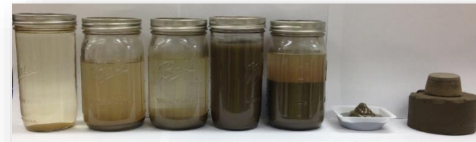
Samples showing a progression of concentration of FGD blowdown at a southern US power plant with the sample on the far right representing a solidified and stabilized residual block with superior mechanical and leaching properties for disposal. Fly ash was used as the stabilizing agent.
