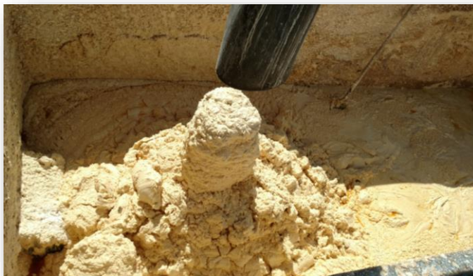
Solids exiting a centrifuge chute at a midwestern power plant. The centrate return from the centrifuge is re-processed in the Concentrator to yield a ZLD solution.
