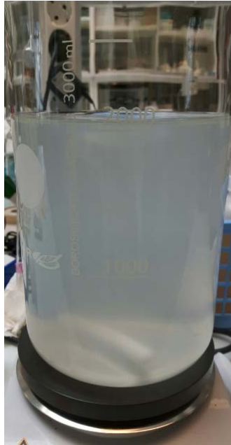
Polymer (400 ppm) dissolved in brine
