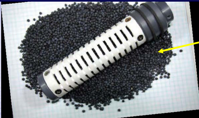
Bio-Trap® Sampler with Bio-Sep® Beads
