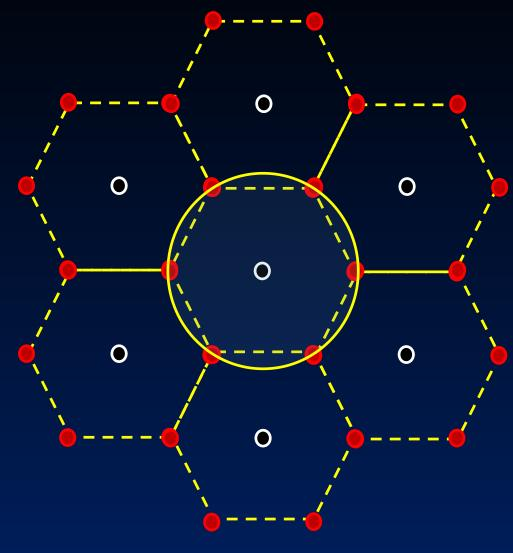
Model simulates removal from a cylinder with no flow boundary and central sink
