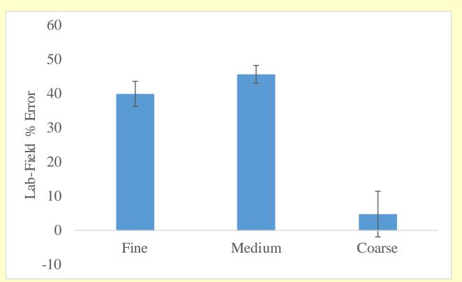
Lab-Field % Error = ((Lab EC - Field EC)/Lab EC)\*100
