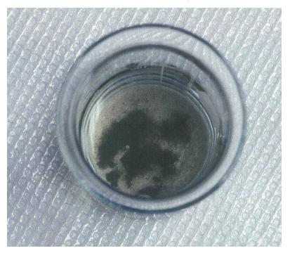
Core Immersed in Bridge Creek 3% KCI Water
