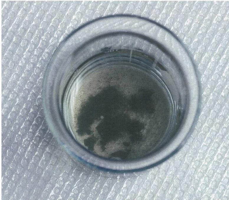
Core Immersed in Bridge Creek 3% KCl Water
