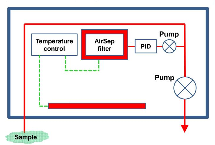
A second heater accurately controls the temperature of the Benzene separation (Air-Sep) filter tube.
