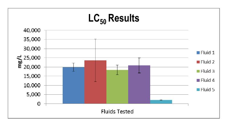
\*EPA WET 2000 was used to test fluids 3 times. Averages and standard deviations are shown.
