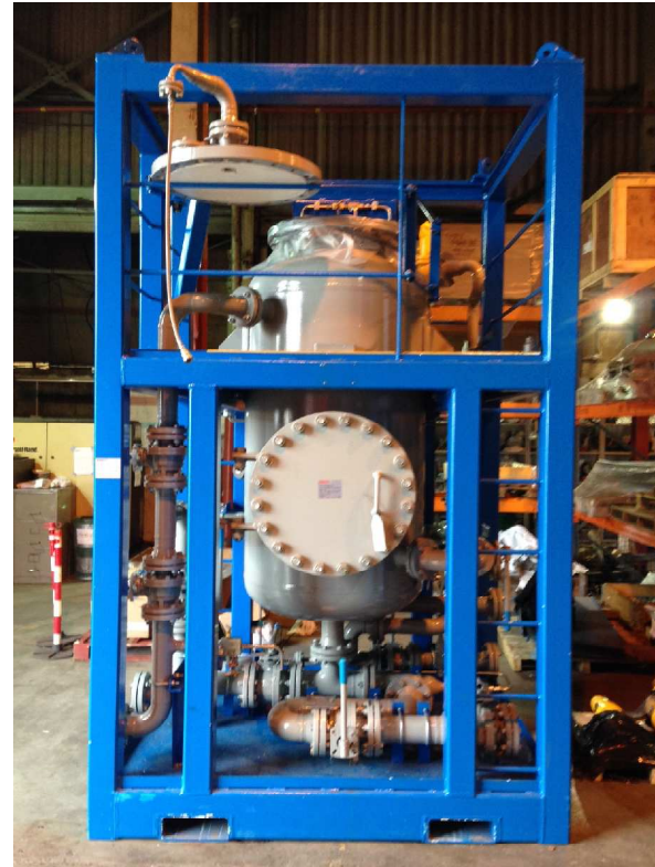
Final polishing for overboard discharge and reinjection
