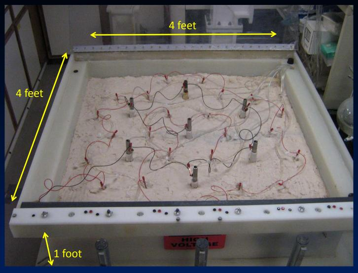
Sodium loading = 500 mg/kg, kaolin clay
