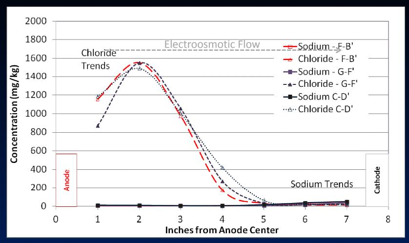
Final bulk sampling results = 83% removal of sodium, 71% removal of chloride
