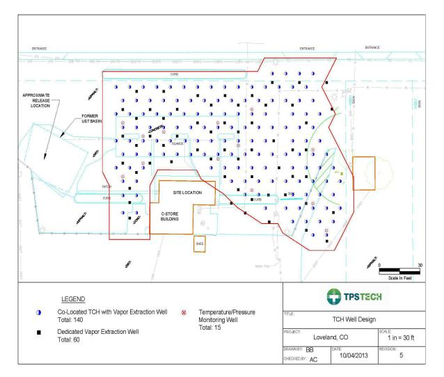
System design includes 140 Thermal Conductive Heating (TCH) wells to supply heat to 14 feet bgs. 70 wells are GTR + F<sup>™</sup> re-heat wells. 140 co-located and 60 dedicated SVE wells. 16 temperature and pressure monitoring points.
