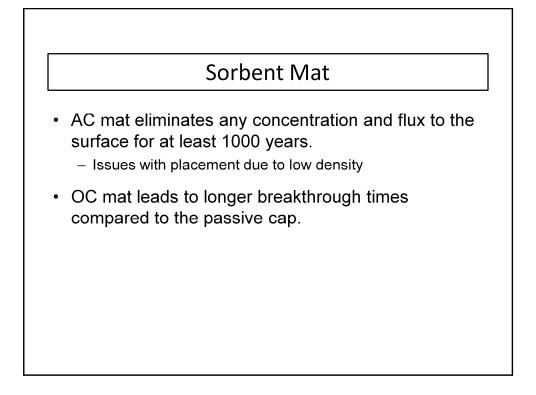
• 1cm mat leads to longer breakthrough times compared to the 30 cm sand only cap although steady state fluxes (after several hundred years) are higher due to the thinner cap thickness in this simulation.
