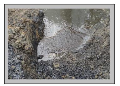
Approximately 2 1/2 inches of viscous free product (light oil, diesel fuel, and gasoline) were present.
