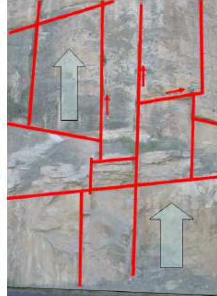
Type 3: Flow in Fractures and Matrix, Storage in Matrix (Dual Permeability)
