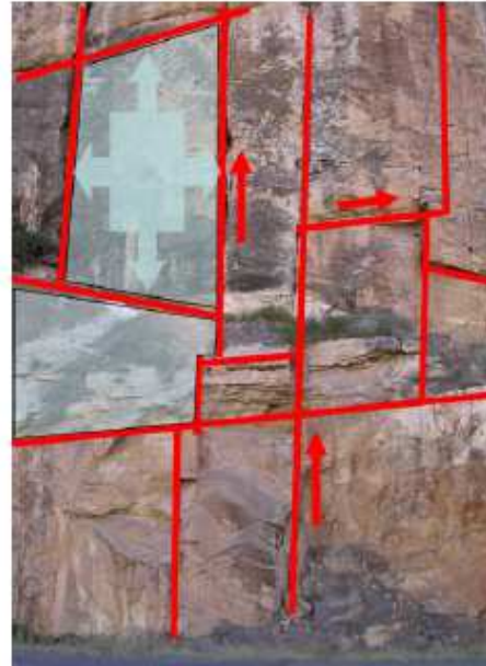
Type 2: Fracture Flow Only, Matrix Storage (Dual Porosity)
