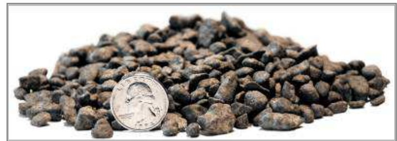
AquaBlok/AquaGate+ “composite particle”
