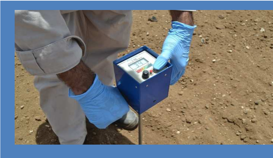
On site Moisture Check & lab Oven for moisture analysis
