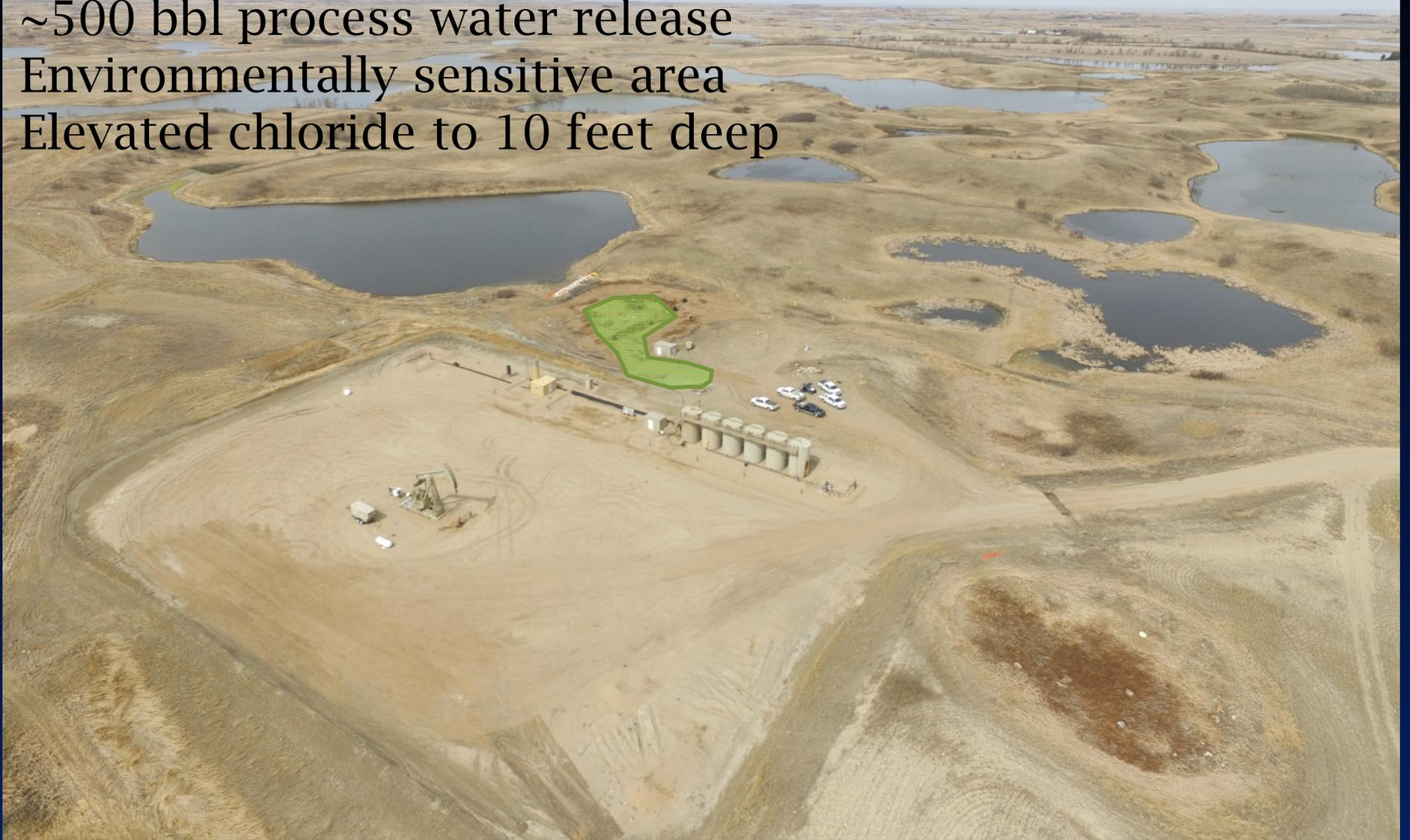
First action was to isolate the small slough from larger, begin pumping affected water from the small slough, and excavate contaminated soil around release point and above the slough.
