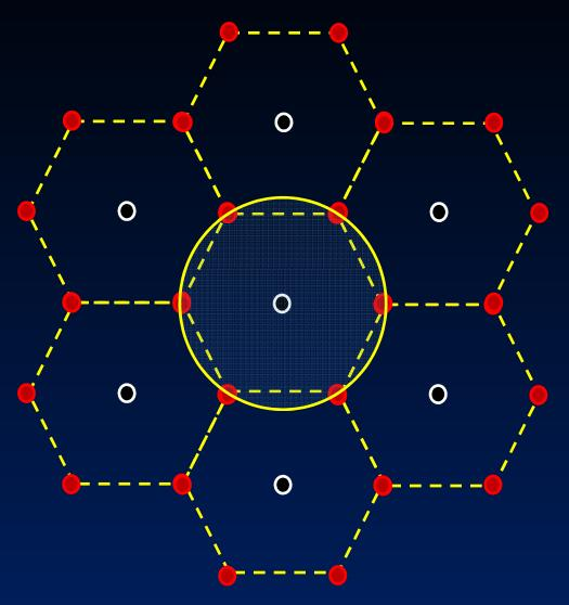
Model simulates removal from a cylinder with no flow boundary and central sink
