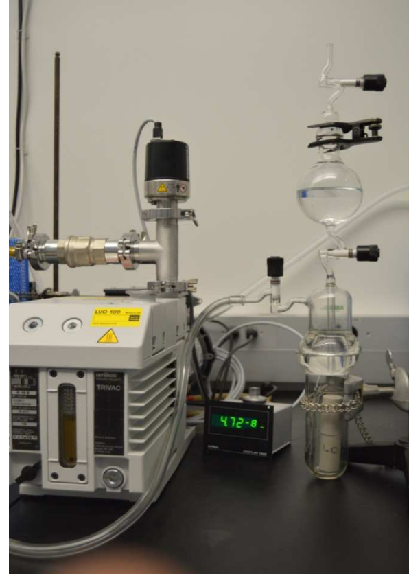
Vacuum pump and cell (100% water saturation)
