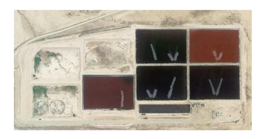
Wright Facility under construction 2016, includes GCL, and double geomembrane with leak layer in between:
