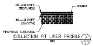
**High Density** Polyethylene (HDPE) designed as the primary or top layer of the lined ponds in order to protect the groundwater and to enhance the evaporation of the production water within the ponds.
