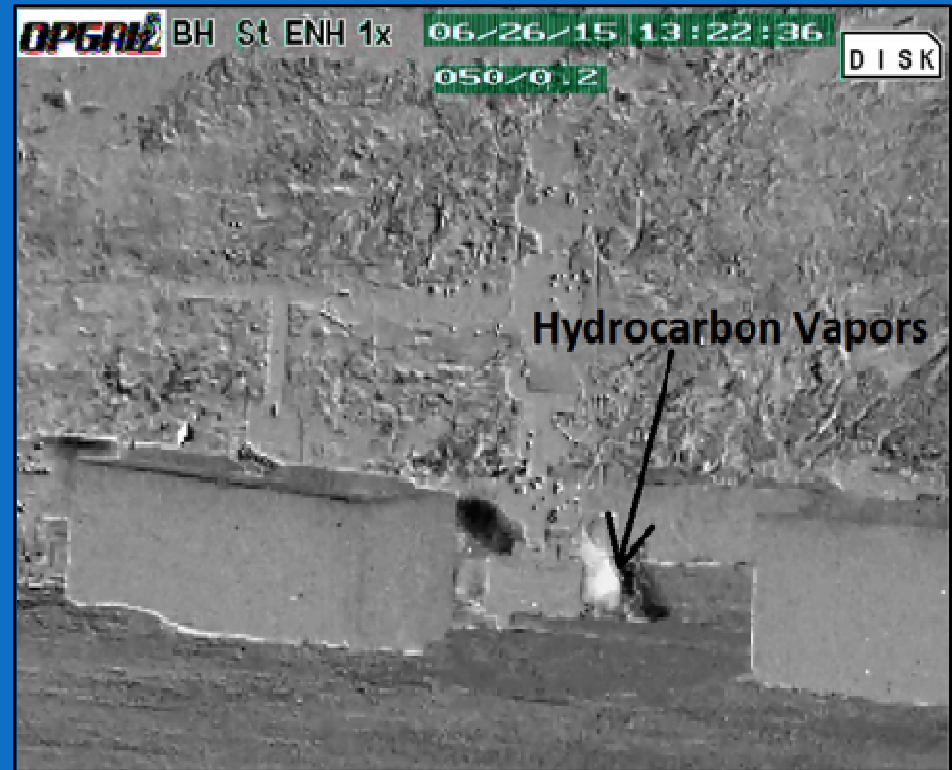
Hydrocarbon vapors are visible in infrared
