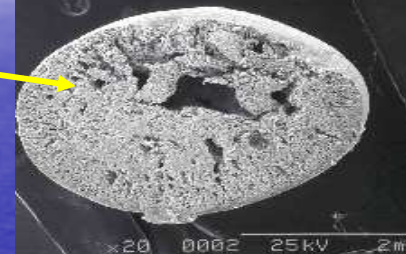
X-Section of Bio-Sep® Bead
