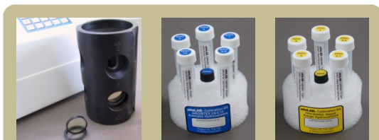
Sitelab's UVF-3100 analyzer has optical filters sensitive to GRO and EDRO range hydrocarbons
