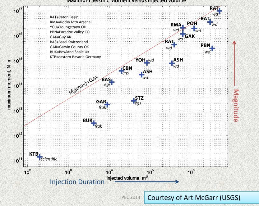
Maximum Seismic Moment versus Injected Volume
